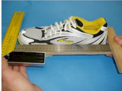
Measurement of footwear length using custom built Brannock-style device
